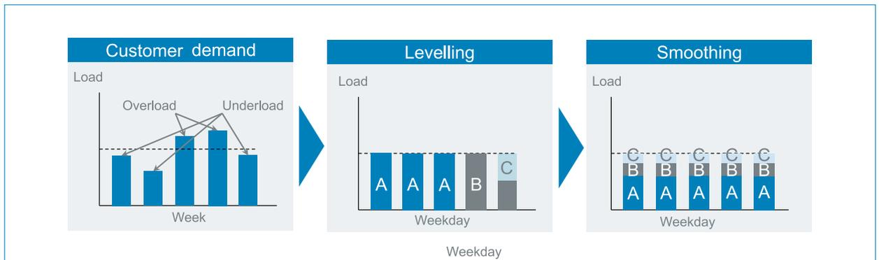
Fig. 10: Mode of action for the levelling and smoothing of customer demand
