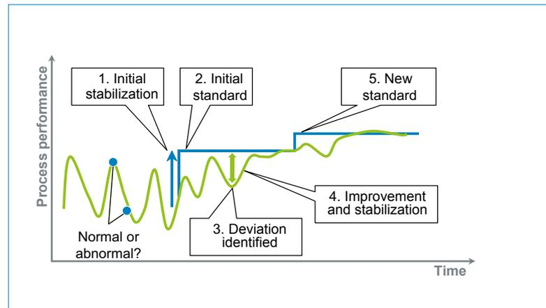
Fig. 8: Connection between stabilization, standardization and improvement
