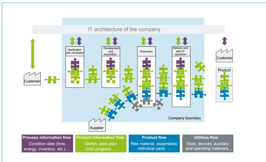
Fig. 18: The integration and synchronization of all information flows creates flow in value stream 4.0
