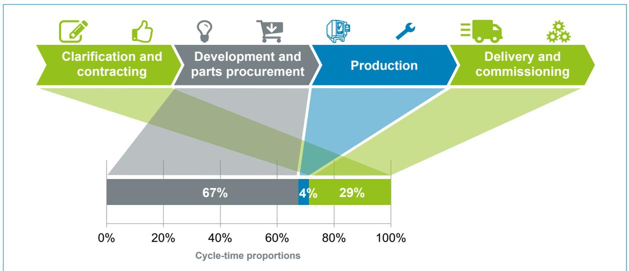
Fig. 13: Assessment of the throughput time proportions from the initial customer contact to the commissioning of a system (example taken from a company in plant engineering)
